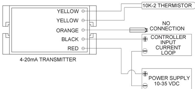
**Fig. 10:** Typical Thermistor 4 to 20mA Transmitter
