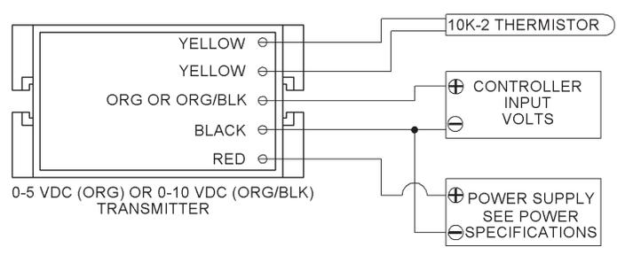
**Fig. 11:** Typical Thermistor Voltage Transmitter
