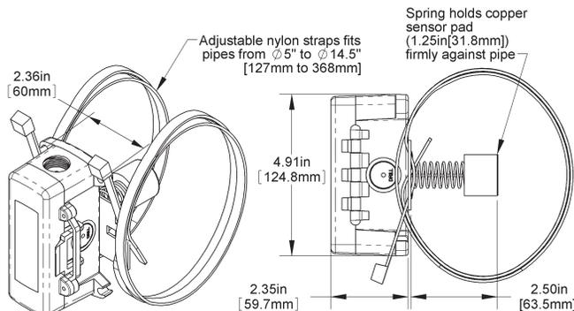
Fig. 5: Spring Loaded Strap Unit in a BAPI-Box 2 (BB2) Enclosure
