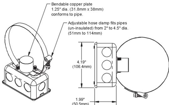
Fig. 1: Clamp-On Strap Unit with Junction Box (Standard)
