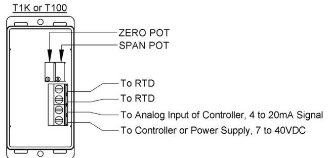
**Fig. 9:** Typical RTD 4 to 20mA Transmitter with Terminals
