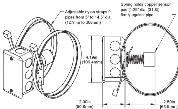
Fig. 4: Spring Loaded Strap Unit in a Junction Box (Standard)
