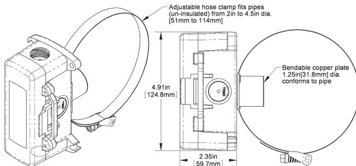
Fig. 2: Clamp-On Strap Unit in BAPI-Box 2 (BB2) Enclosure
