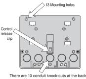
and bottom of the wiring chamber.
