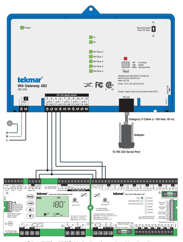
Refer to W422 and W337 wiring brochures for complete wiring schematic.
