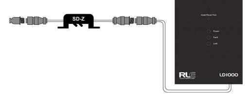
If the SD-Z is being added to an existing system - connected in a chain with other SD-Z devices or cable - undo the appropriate coupling, insert the SD-Z into the chain, and secure all connections.
