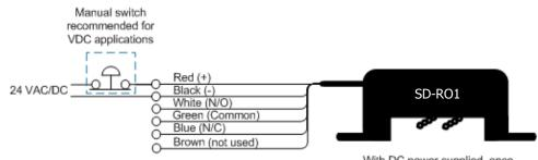
With DC power supplied, once triggered, SD-RO1 latches on until power is manually removed
