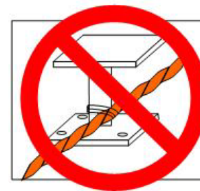
Secure to pedestal with tie wrap. Do Not Secure as Shown
