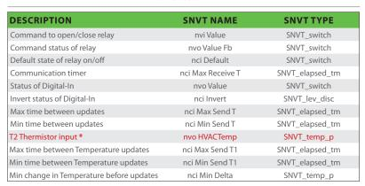
The relay will go to the default state when the communication timer times out. Setting the timer value to zero will cause the communication to never time out.
