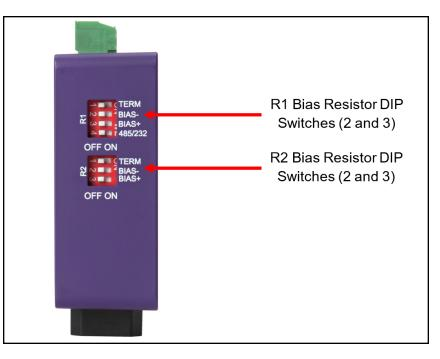
To enable Bias Resistors, move both the BIAS- and BIAS+ dip switches to the right in the orientation shown above.
