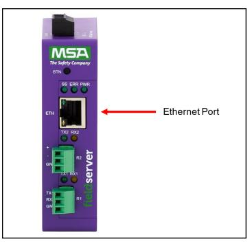
The Ethernet Port is used both for BACnet/IP communications and for configuring the QuickServer via the Web App. To connect the QuickServer, either connect the PC to the Router's Ethernet port or connect the Router and PC to an Ethernet switch. Use Cat-5 cables for the connection.
